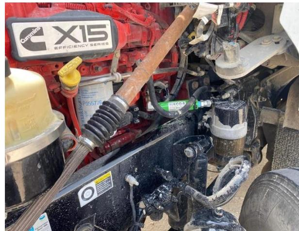
The ECO#5 is illustrated and installed in the middle of the primary and secondary fuel filter
